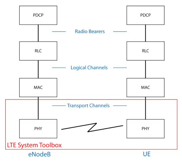
LTE System Toolbox focuses on the physical layer, which is highlighted in red in the preceding figure. It also supports interfacing with portions of the RLC and MAC layers, which are highlighted in blue. The primary features of the LTE physical layer are OFDM
