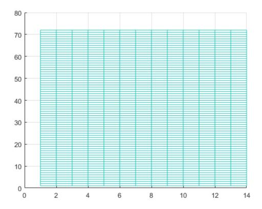
After the indices are generated and the reference symbols are mapped to the resource grid, the resource grid is replotted to show the reference symbol mapping.
