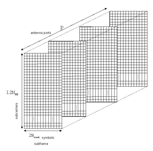
The rows of this array represent the subcarrier. The columns map the OFDM or SC-FDMA symbols in the downlink and uplink, respectively. The third dimension or plane represents the antenna ports. In the LTE System Toolbox, the resource grid spans a subframe in the time-domain, instead of a slot. Hence, the documentation uses the term
